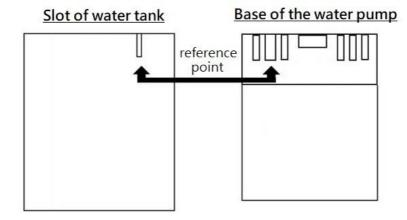
2. With reference to the above illustration, align the reference point of the water pump base to the slot of water tank.
