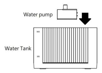
1. After cleaning the water pump, place the pump on the slot inside the water tank.
