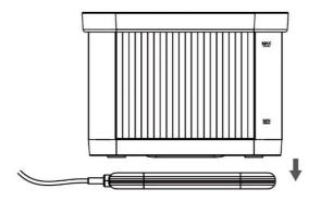
3. After assembling the water tank and all accessories, place the water tank on top of the USB power base.
