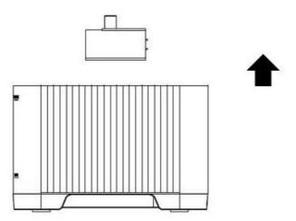
Lift up the upper lid of the water tank and take out the water pump. Pour out all remaining water inside the tank.
