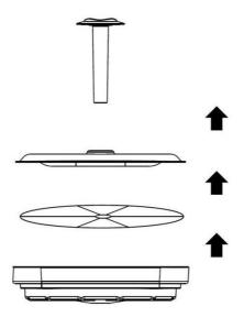
1. Take out the outlet pipe and metal water tray in order to replace the filter core.
