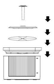
Install the upper lid, filter core, metal water tray and outlet pipe on top of the water tank one by one. The assembly of accessories is finished
